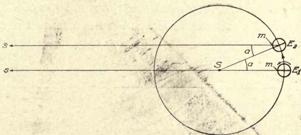
Fig. 44. The Solar Days Are about 4 Minutes Longer Than the Sidereal Days Because the Earth Revolves around the Sun
